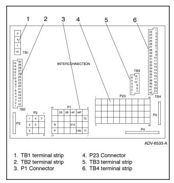
Figure 1-10 Interconnection Circuit Board Terminal Strips and Connectors
